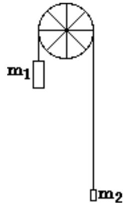
1. A 200-gram and 50-gram mass are connected by a string stretched over a pulley. Determine the acceleration of the masses and the tension in the string.
