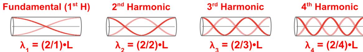
2<sup>nd</sup> Harmonic: one-half the  $\lambda$  of 1<sup>st</sup> Harmonic ... and two times the  $f$ .
